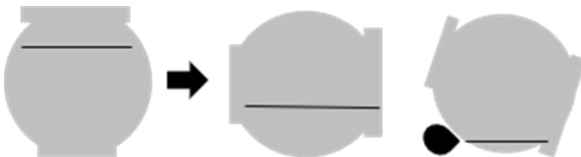
Effect of tipping on water level.
